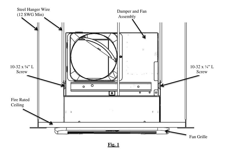
For fan models: SMT130, SMT130H, SMT130M, SMT150, SMT150D, SMT150LED, SLM80 and SLM100.
